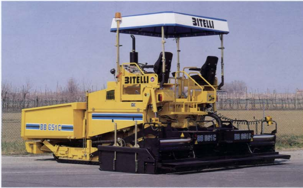
Paver finisher BB 651 C fitted with folding canvas canopy (item on request)
